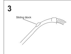
You can adjust the airflow by push the sliding
