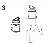
Press the automatic release button to empty the dust into dust container.
