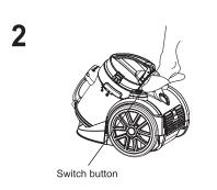
Press the switch button to turn on/off the cleaner.
