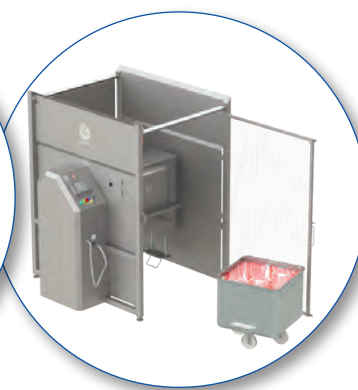
Trolley with the finished batch discharged for further processing
