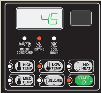
**Quantum™ Control Features:** Digital display for vend price and cycle time countdown. Touch pad control with LEDs. Four cycle selections, dedicated Push-to-Start pad. Infrared programming.
