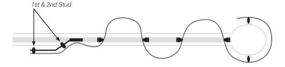
■ For the Master Carrier on a centre open curtain, the 1st and 2nd stud go either side of the master carrier creating a folded edge.
