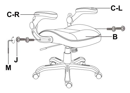
Note: Attach Armrests (C) to the assembled Seat Cushion (B) using 4x Screws (J) with Allen Key (M). **Do not tighten Screws fully until you have completed assembly.**
