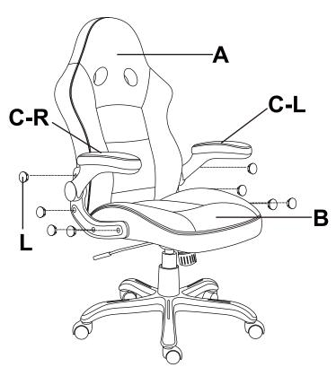
Note: Fully tighten all Screws (J) with Allen Key (M). Press the Plastic Caps (L) into the Armrest holes to cover the screws.
