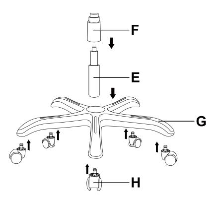
Note: Turn the Star Base (G) upside down. Push the Castors (H) firmly into hole at the end of each leg. Turn the Star Base (G) upright and insert Gas Lift (E) into the center hole of Star Base (G). Place cover (F) over the Gas Lift (E).
