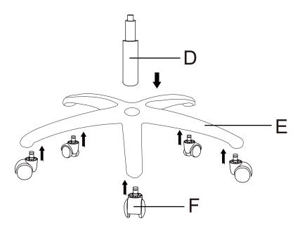
Note: Turn the Star Base (E) upside down. PUSH the Castors (F) firmly into hole at the end of each leg. Turn the Star Base (E) upside and insert Gas Lift (D) into the center hole of Star Base (E).
