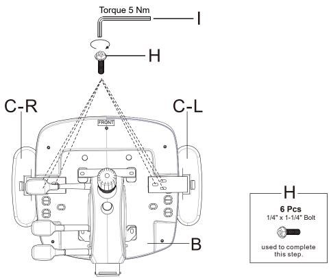
Note: Attach Armrests (C) to the Seat Cushion (B) using 6x Screws (H) with Allen Key (I). Only applicable for when using a drill. Set torque to 5Nm.
