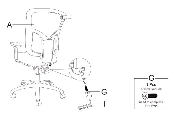
Note: Align Back Cushion (A) with Seat Cushion (B) by GENTLY inserting J-bar into the rear hole of the Seat Plate (B) as shown and TIGHTEN by using 3 x screws (G). Only applicable for when using a drill. Set torque to 5Nm. Before using your Chair, ensure that all the screws are tightened fully for safety.
