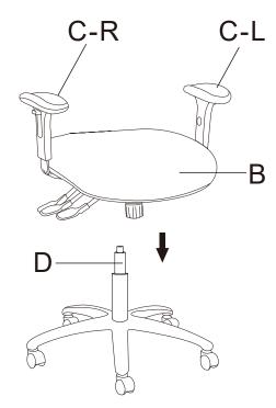
Note: Place assembled seat on the Gas Lift (D). Push down firmly until connection is secure.
