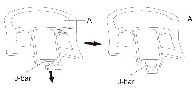
Note: Extend the J-bar by holding the backrest with one hand and pull the bottom of J-bar with other hand.
