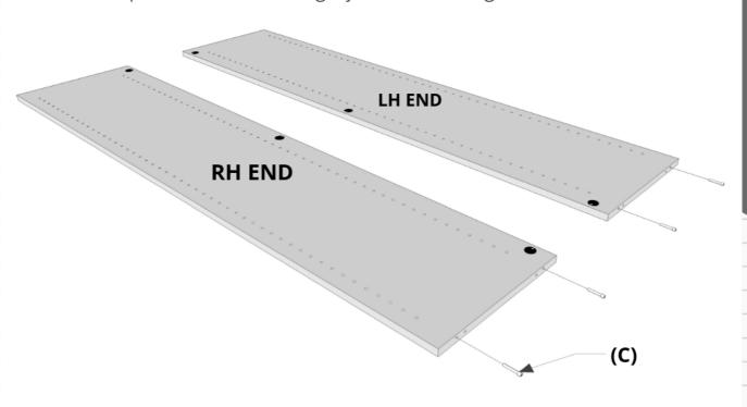
Take your two (2) METAL DOWELS **(L)** and slide into central pre-drilled holes to join the left hand side (LHS) and right hand side (RHS) back panels together.
