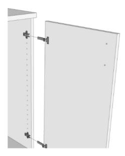
**NOTE:** You can adjust your doors using the 2 screws located on your hinge. The back screw adjusts the door forward or back. The front screw adjust your door left or right.
