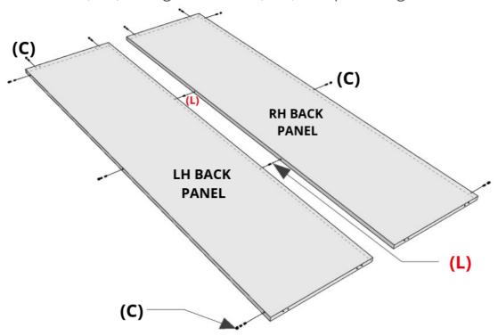
Then insert ten (10) PINS (C) into the outer pre-drilled holes on the back panels with your screwdriver.
