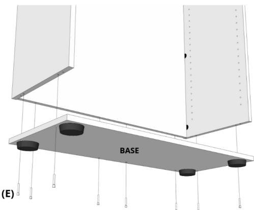
**NOTE**: On un-even floor the two part foot can be adjusted out to level the bookcase.
