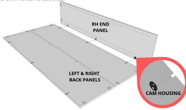
Fix the bookcase top to the back & ends by aligning the PINS (C) with the preinserted CAM HOUSING and tighten by rotating the CAM HOUSING screw clockwise using your screwdriver.
