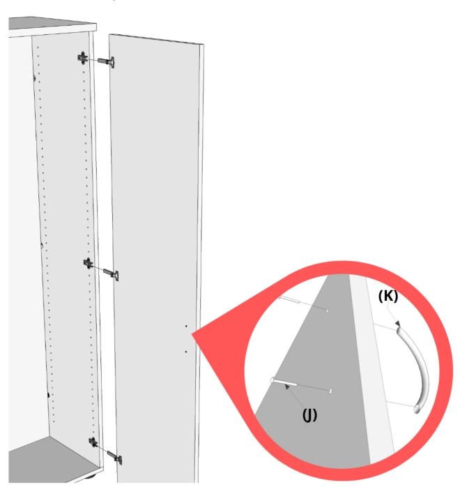
Align door hinges with hinge plates. Hook front section of the hinge to the hinge plate then push the back of hinge until it clicks in place and is secure.
