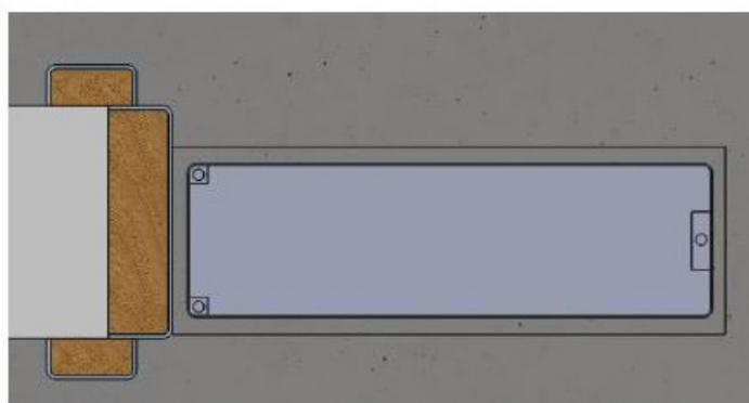
8. Once the housing is located properly, fill the surrounding area with quick drying concrete.
