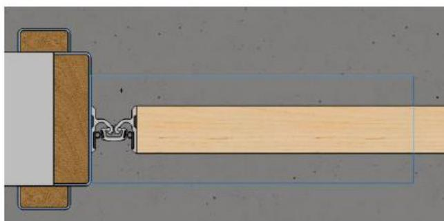
6. Remove the closer from the housing by unscrewing the 3 locking screws. Once they are loose, the closer should slide out.
