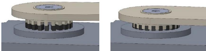
17. Carefully unscrew the 180° - 15° screw, tightened in step 12, and the door will begin to close. **DO NOT USE AN ELECTRIC DRIVER.** This screw is used to set the closing speed. **DO NOT FULLY UNSCREW** as this will cause hydraulic fluid to leak and **PERMANENTLY** render the product inoperable. Refer to the setup pages for final setup method.
