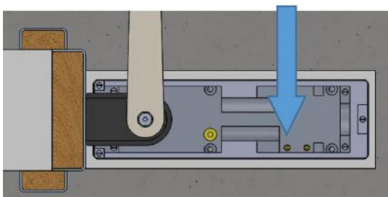
14. Mark the Location of the closer on the closer body then remove the closer arm. This mark is needed later when the arm is re-fitted.
