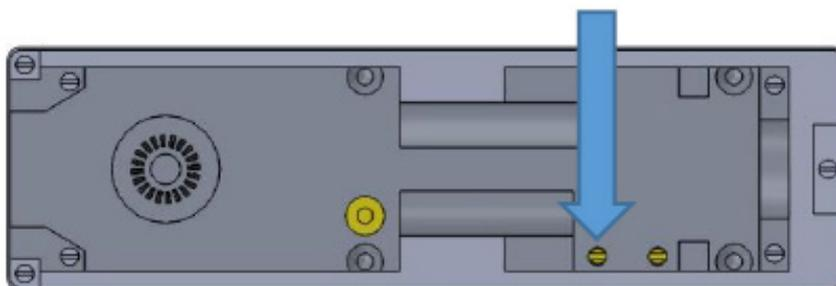
3. Tighten 0° - 15° [Latching speed] screw until it begins to tighten.
