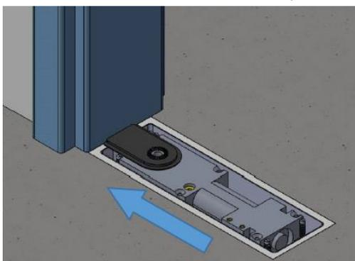
10. Use the 4 adjustment screws to fine tune the positioner, making sure the main body is flush with the floor.
