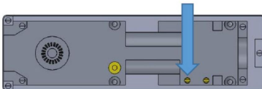
2. If the latching function is too soft to latch the door fully, begin to unscrew the latching speed screw. This should be adjusted 1/4 turn at a time. **Do not fully unscrew this as the closer will be rendered inoperable permanently.**
