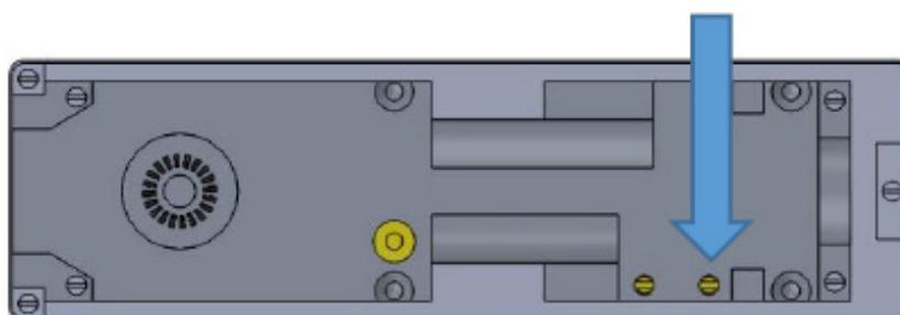
2. Test the operation, if the latching is now functioning then adjust the screw by unscrewing [anti-clockwise] it until the desired latching speed is achieved. Follow the setup instruction.
