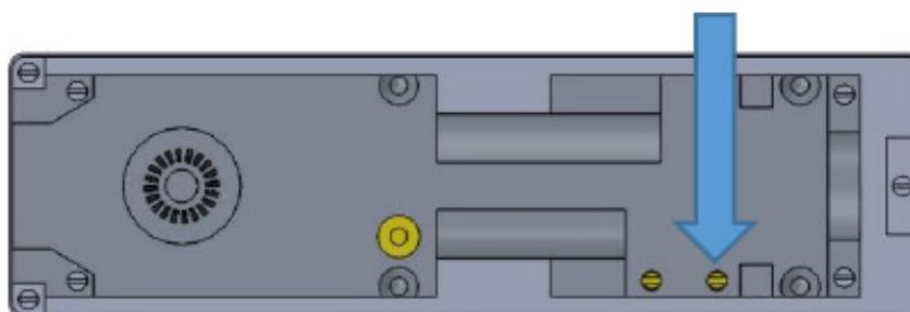
1. Unscrew the closing speed screw until the door begins to close. Keep unscrewing until the desired closing speed is achieved. This should be adjusted at 1/8 turn at a time. **Do not fully unscrew this as the closer will be rendered inoperable permanently.**
