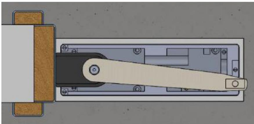
13. Open the arm to roughly  $90^\circ$  in the direction the door will open, this will require a lot of force. Lock the arm in place by carefully, slowly, tightening the  $180^\circ - 15^\circ$  screw fully clockwise. **DO NOT USE AN ELECTRIC DRIVER**
