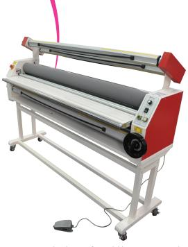
The economical solution for cold laminating and mounting to 1600mm wide and 32mm thickness. Incorporating a product feed/backing film delivery system, this machine represents outstanding value and simplicity that delivers an expert finish with no experience necessary.
