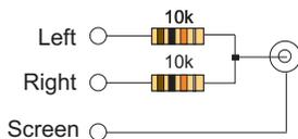
Ideally fit the two 10k, 1/4W, summing resistors within the body of the jack plug
