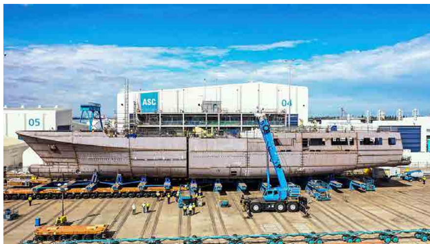
Figure 3.2: The two halves of the first offshore patrol vessel being joined together in May 2020
