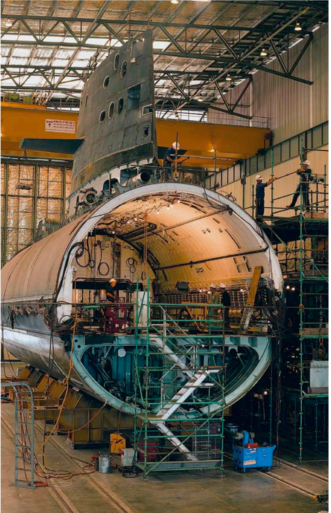
A Collins submarine in build at the Australian Submarine Corporation. Courtesy of ASC Pty Ltd
