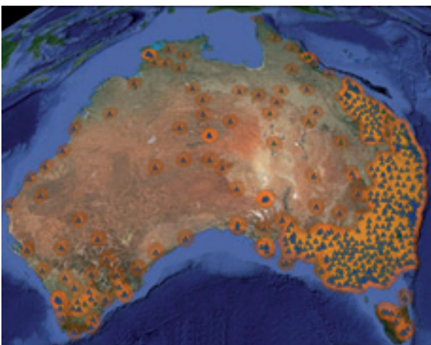
Each orange circle represents a RTK reference station. As of December 2013, the network comprised of more than 500 base stations.
