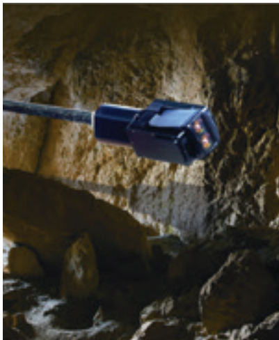
Underground cavity scanning with the Optech CMS-V400 scanner.
