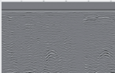
Road culverts at 6 meter depth
