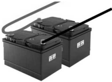
Figure 5: Recommended wiring for connecting batteries in parallel.
