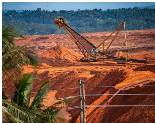
Sand stackers backfilling mined out Central Dune
