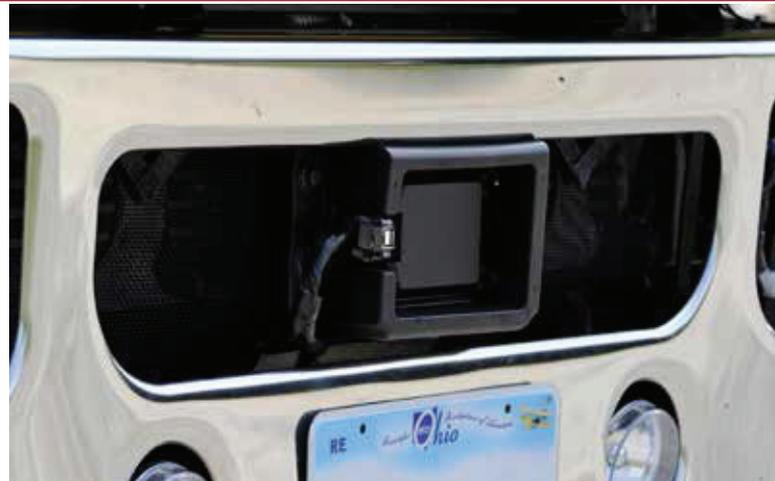
**Advanced radar system offering superior adaptive cruise control that is reactive to provide higher braking efficiency to minimise risk of collision.**
