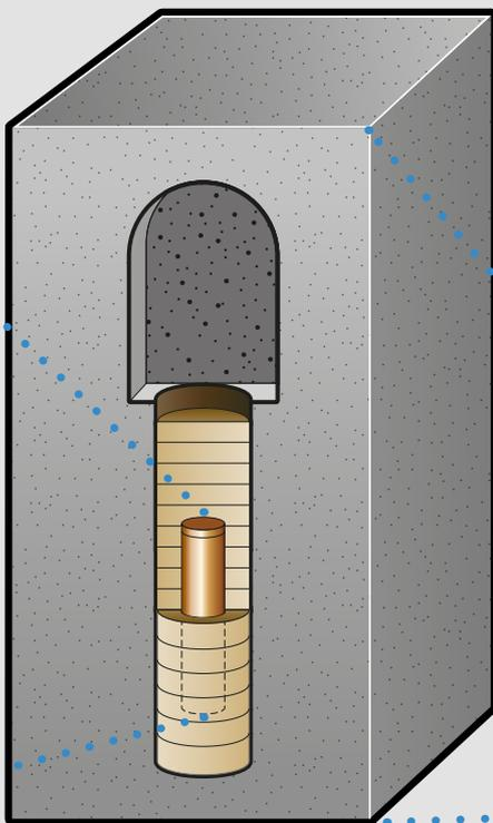
Bentonite buffer and tunnel backfill
