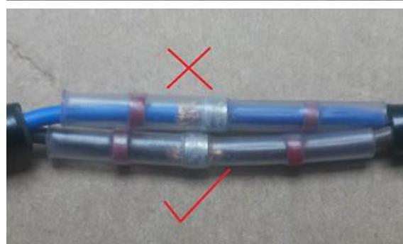
7. Using a heat gun on Medium to High heat, gently heat the centre of the solder splices until the solder ball melts and runs into the wire. Take care to only heat around the solder ball as excess heat can damage the cable. Check that the red seals next to the solder balls have also melted.
