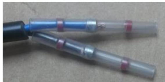
6. Slide the wires from the new cable into the solder splices and position each splice so that the silver coloured solder ball is positioned over where the 2 wires join.
