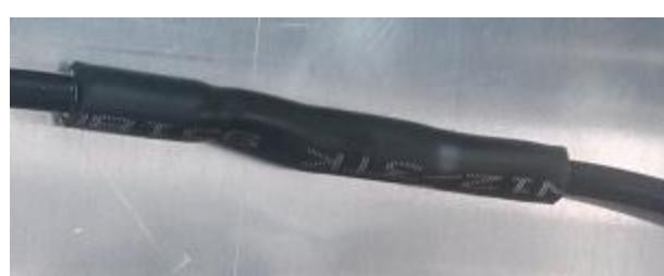
10. Once the heat-shrink tube has shrunk completely the glue from inside of it should be visible on the ends.
