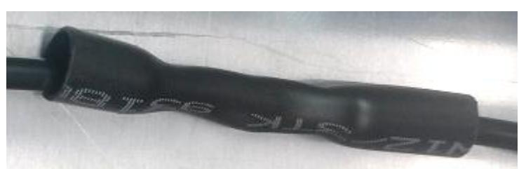
9. Continue heating the heat-shrink tube towards the ends but be CAREFUL not to heat the cables directly as they can be DAMAGED.
