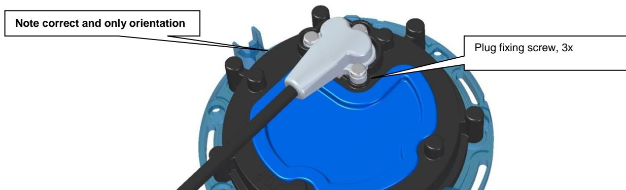
4. Double check that the cable gland inside the niche is tightened. Coil the remaining cable into the niche, leaving enough spare cable in the niche to be able to bring the light (with cable attached) above the waterline. This allows for easy servicing at a later date.
