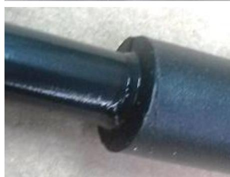
11. Leave the completed joint to COOL for 5 minutes to ensure that the glue seal isn't damaged. Once cooled, momentarily power the light to confirm that the connection is sound.
