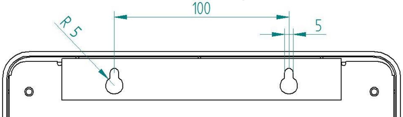
2. Hang the SLX Lighting Transformer from the two screws, ensuring that the power supply drops down into place and is locked in position. Plug the SLX power supply’s mains cable into a mains outlet.
