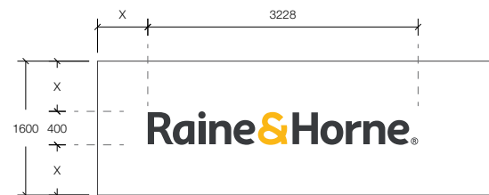
TR-400-N - Transom Lettering + TRANSOM-1600-(AorB) - Transom Cladding *400mmH logo to applied to transoms between 1401-1600mmH
