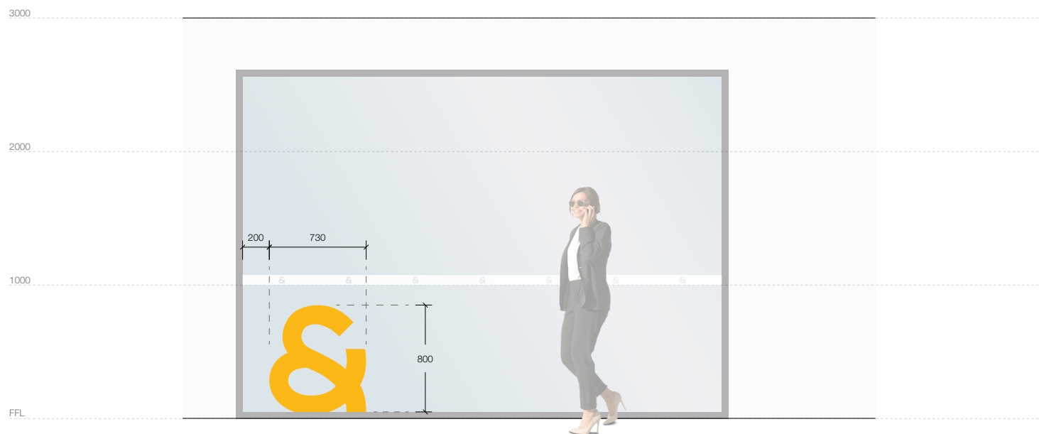
Typical Elevation - Ampersand - Low Level Scale 1:25
