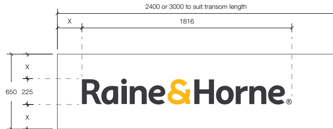
TR-225-N - Transom Lettering + TRANSOM-650-(AorB) - Transom Cladding *225mmH logo to applied to transoms between 600-800mmH
