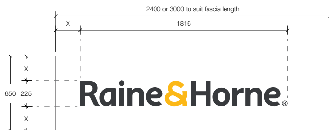
■ FA-225-N - Fascia Lettering + FASCIA-650-(A,BorC) - Fascia Cladding *225mmH logo to applied to fascias between 600-800mmH
