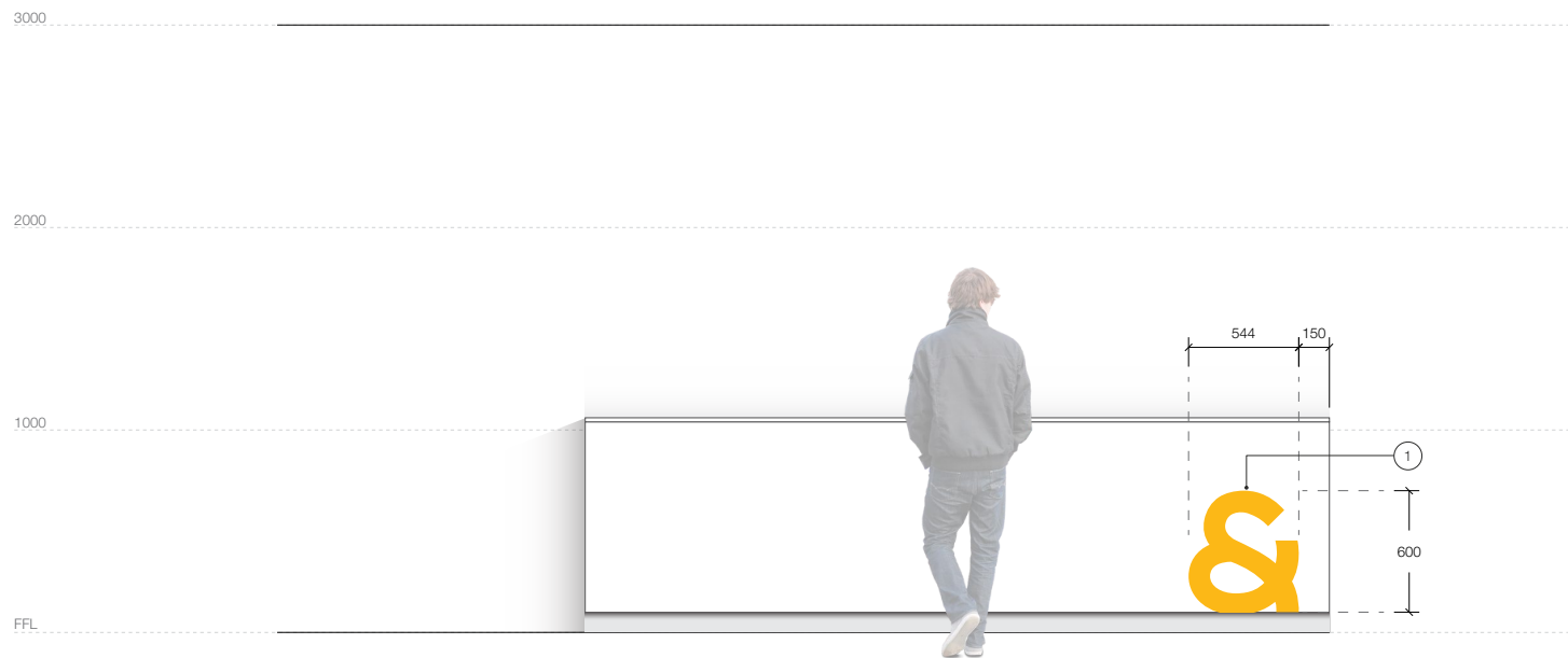
Typical Reception Desk Elevation Scale 1:25
