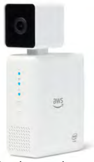
DeepLens – a deep learning-enabled wireless video camera.
