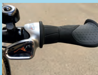
The throttle-like gear changer (middle) with the display showing selection for an incline.
