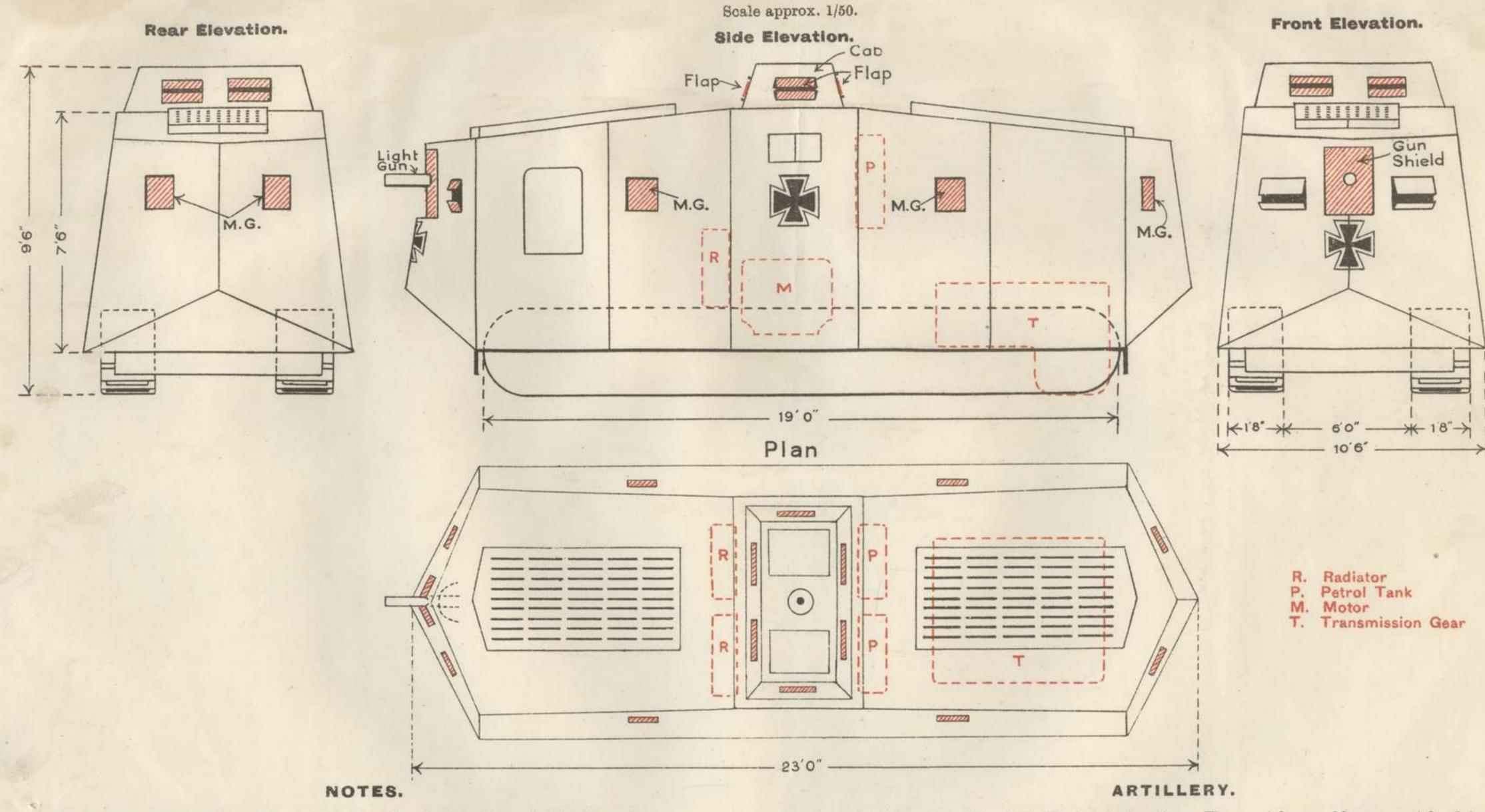
Points most vulnerable to Rifle and Machine Gun bullets shown hatched in red.
