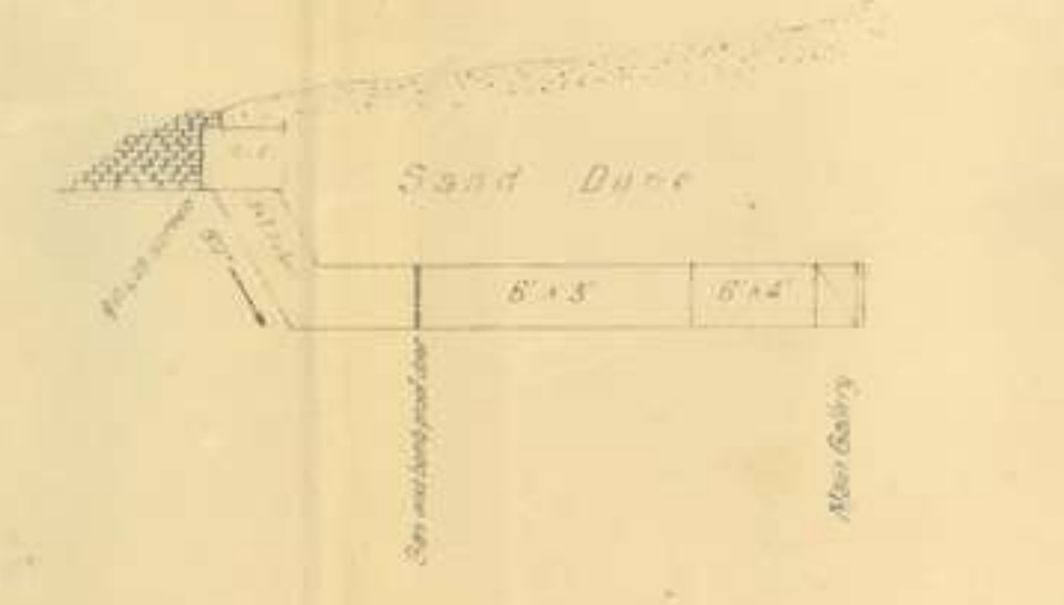
Typical Section where Inclines are used Scale 1 in to 20 ft
