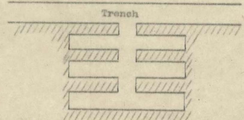
"This will accommodate 6 to 8 men, one in each recess and 2 in the "entrance passages. Digging a dugout of this design with a 3 feet "tunnel would require 306 cubic feet of earth to be excavated or "38.25 cubic feet per man accommodated; whereas one to hold 6 men of the other design (12 feet by 6 feet) would take 246 cubic feet of excavation or all cubic feet per man accommodated.
