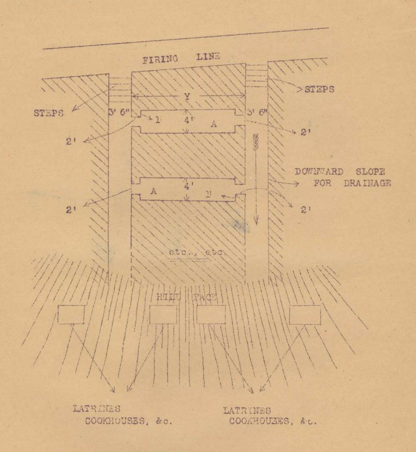
Floors of A. A. to be raised above level of communication trench.
