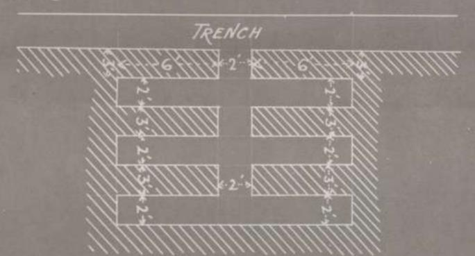
"This will accommodate 6 to 8 men, one in each recess and 2 in "the entrance passages. Digging a dugout of this design with "a 3 feet tunnel would require 306 cubic feet of earth to be "excavated or 38.25 cubic feet per man accommodated; whereas "one to hold 6 men of the other design (12 feet by 6 feet). would take 246 cubic feet of excavation or 41 cubic feet per man accommodated.
