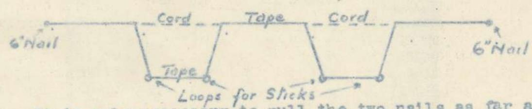
It is only necessary to pull the two nails as far apart as possible, stick them in and then adjust the traverse loops to get a standard fire bayed trench. The operation can be done by two men crawling.
