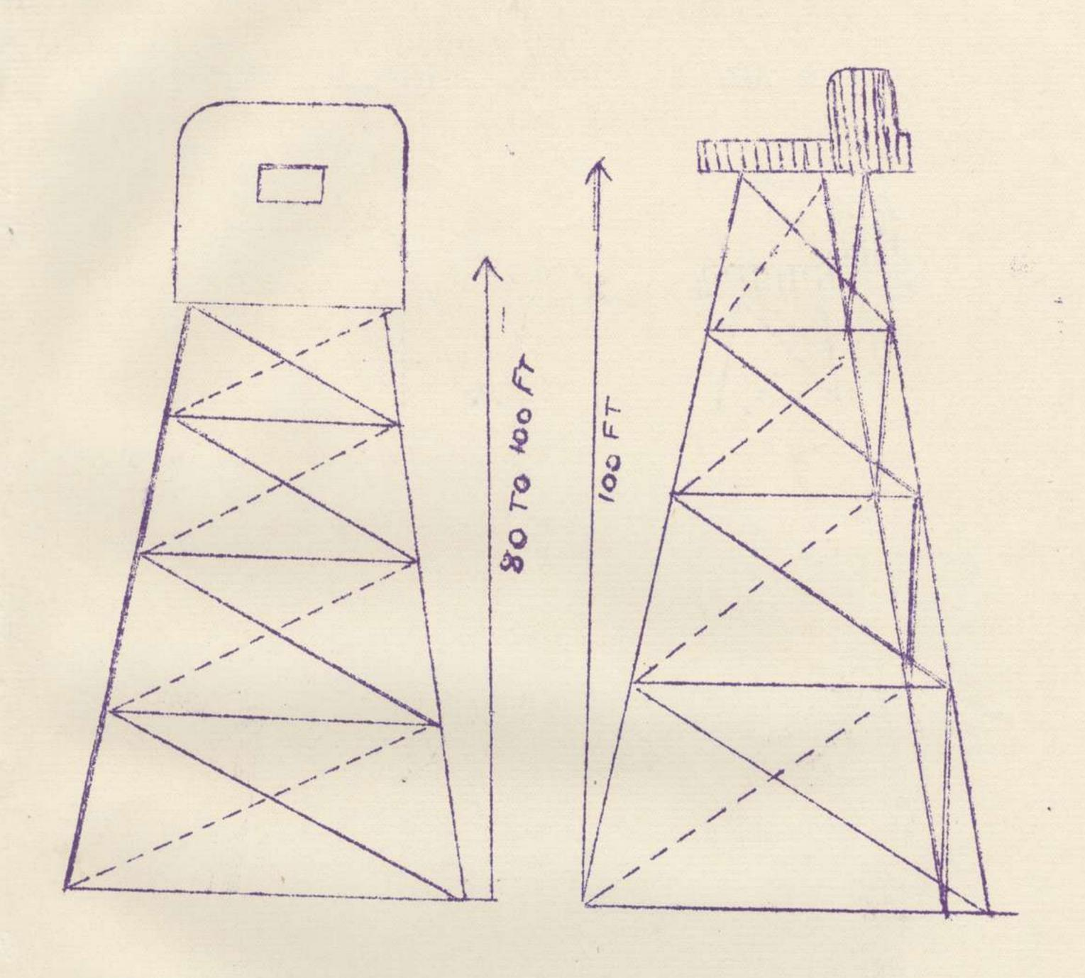
Observing station consisting of a steel skeleton frame-work about 80 ft high, supporting a sheet iron cabin.
