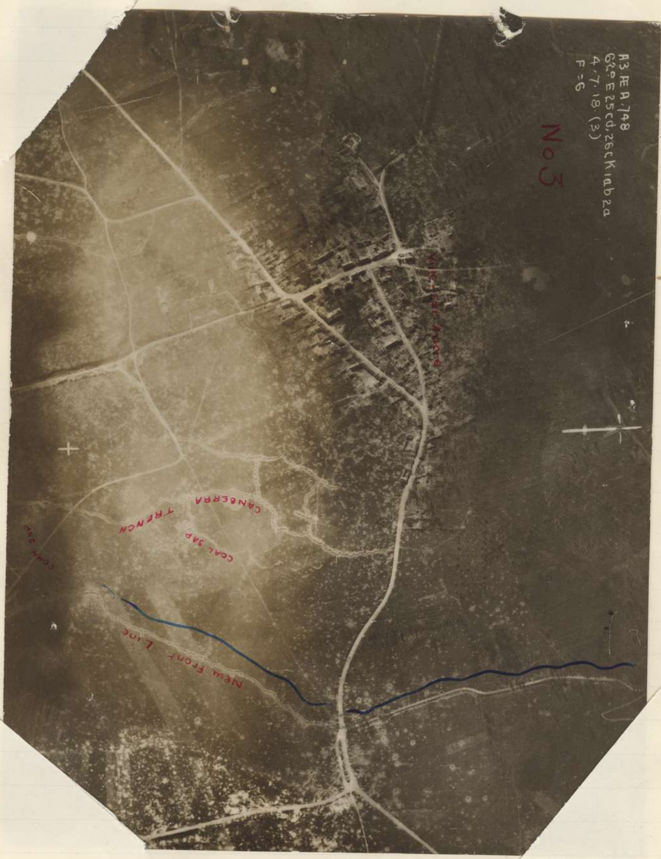
No.3. Shews CORN SAP continued some 40 yards beyond the road also the "T" head at the road. This work was done the night before that of the attack the sap now being only about 40 yards from the enemy line. In this photo COAL SAP is seen connected up with the post.
