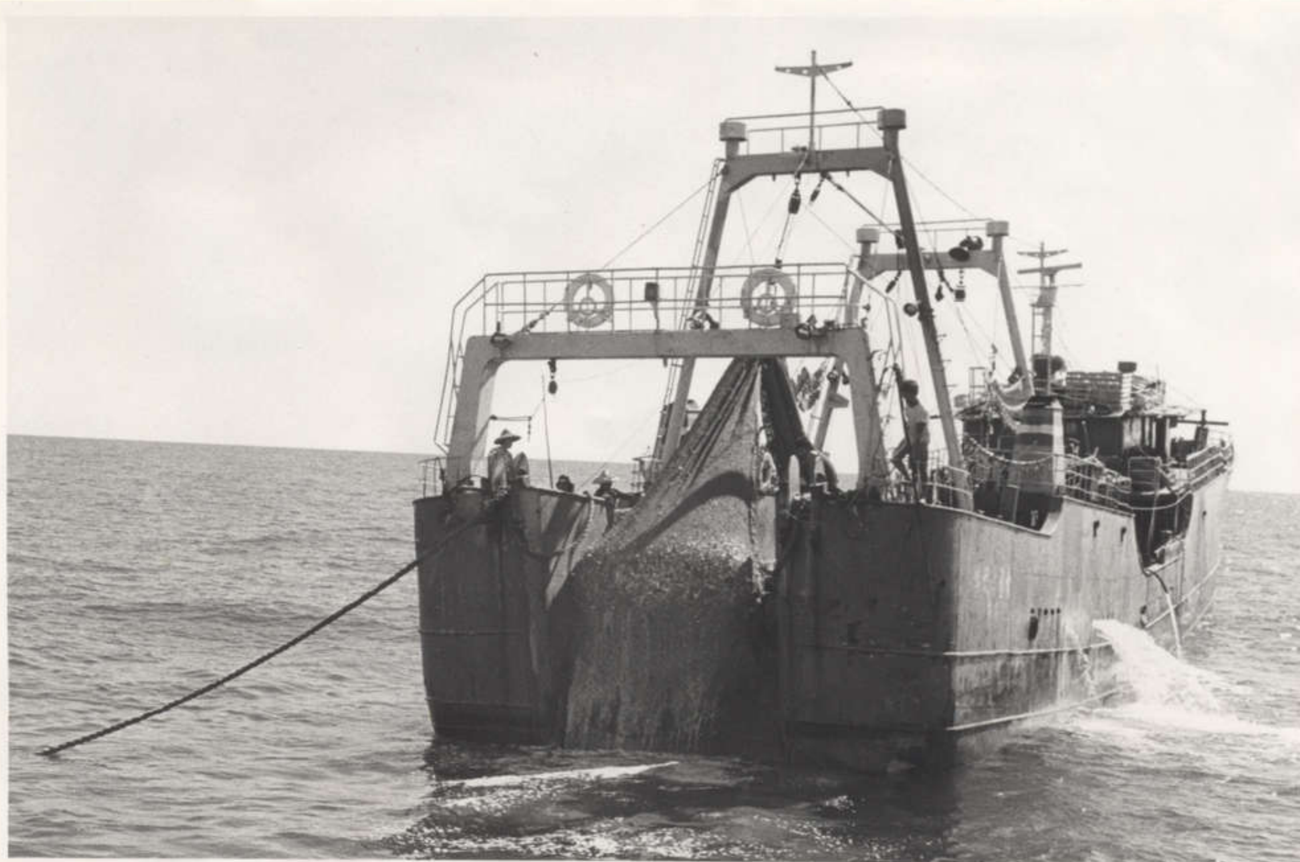
A Taiwanese stern trawler of the type shown above recovering the final portion of the trawl. The hawser for the next trawling net, which will be fed out by the accompanying trawler, has already been passed by heaving line and can be seen leading from the port quarter.
