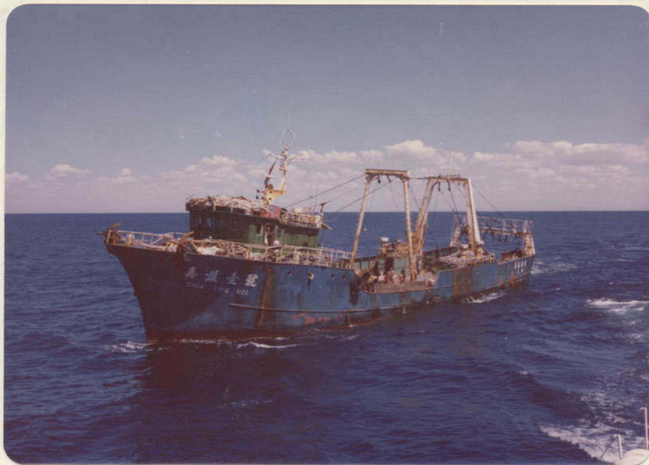
An example of the style of stern trawler most commonly encountered in the Gulf and Northwest Coastal areas.
