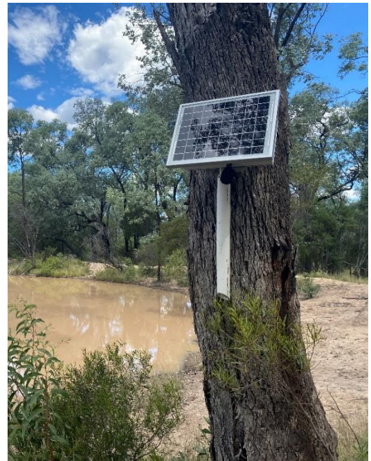
Figure 22 Acoustic recorder setup (G. Young).
