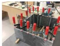
Bond the box to the worktop and clamp into position. Allow adhesive to partly cure, clean off excess and allow to fully cure.
