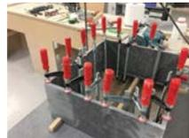
Bond the box to the worktop and clamp into position. Allow adhesive to partly cure, clean off excess and allow to fully cure.
