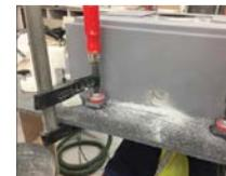
Clamp all blocks until adhesive is fully cured. Drill out overflow hole using 30mm hole saw.
