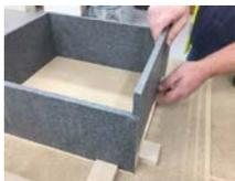
Allow adhesive to partly cure, clean off excess and allow to fully cure. Measure for the remaining two panels to create a box.
