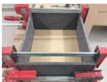
Clamp box whilst curing. Allow adhesive to partly cure, clean off excess and allow to fully cure.
