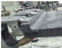
Bond cove strips to panels using Corian® joint adhesive, ensuring the areas are cleaned prior with Industrial Denatured Alcohol (IDA). Clamp cove to panel.
