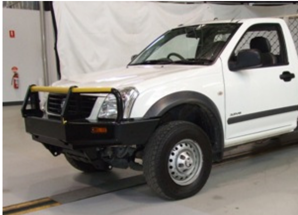
Figure 1. 4WD vehicle fitted with geometrically complying bull-bar
