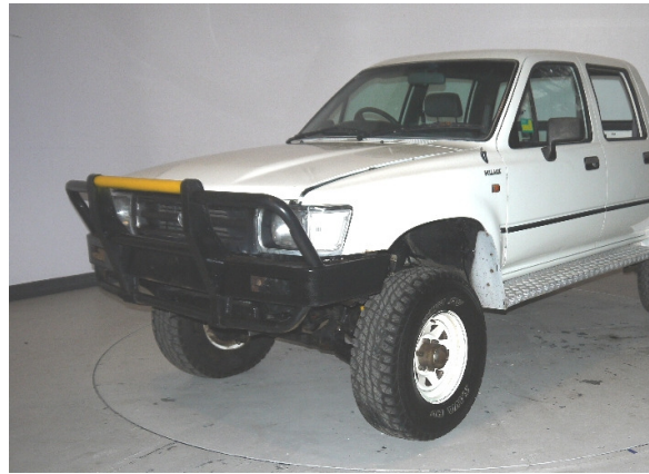
Figure 2. 4WD vehicle fitted with geometrically non-complying bull-bar
