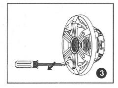
Screw down each of the four Phillips head screws.The locking tabs will swivel into place and secure the unit to the rear surface.Apply the adhesive strip to secure the grill.
