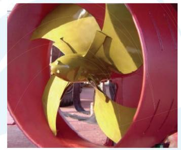
Propspeed can be used on any size boat, from a small yacht to a large commercial vessel. This photo is of Propspeed applied to a commercial trawler.
