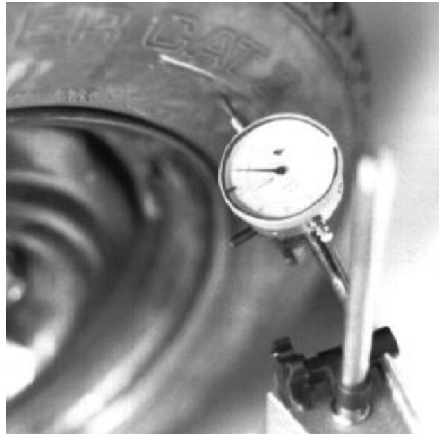
Figure 1.3. Using a dial indicator to check lateral run-out.
