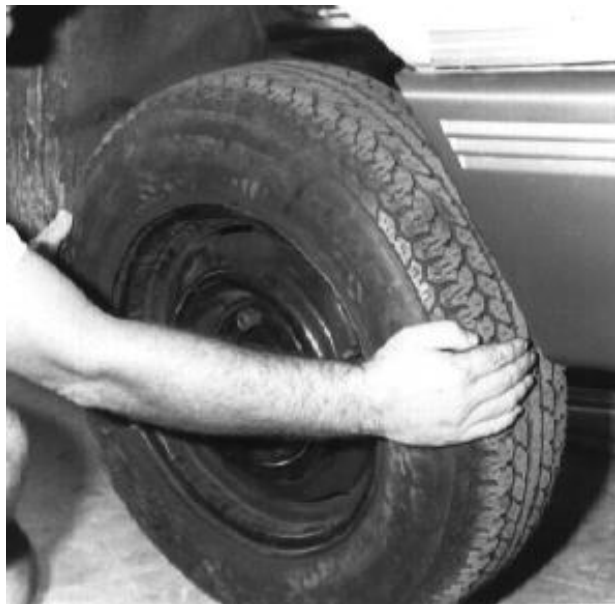
Figure 1.1. Checking wheel bearing end play.
