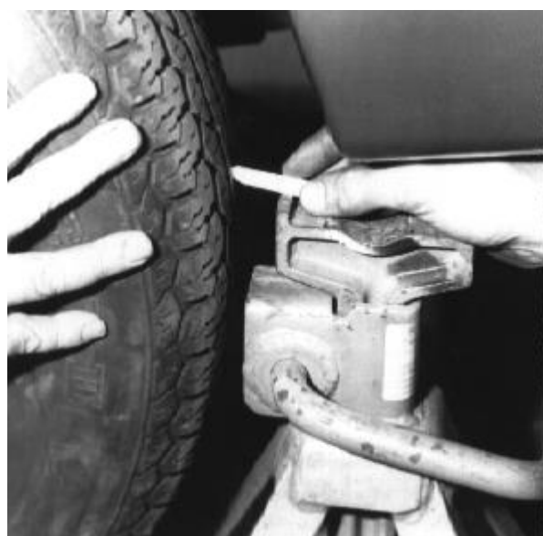
Figure 1.2. Using chalk to check radial run-out.
