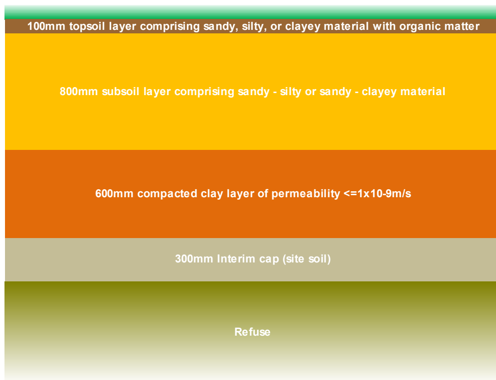
Figure 1 Typical Final Landfill Capping Profile
