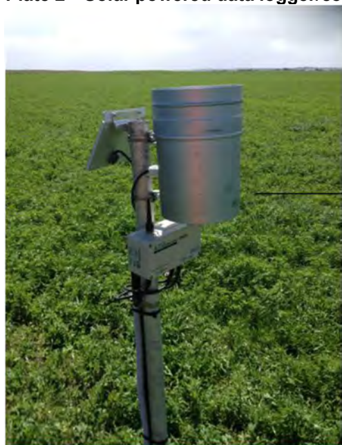
Plate 2 Solar powered data logger/controller with rain gauge
