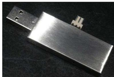
Geosignal XT100 Temperature Logger
