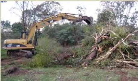
An excavator working with 2 fallers with chainsaws is generally the preferred method for mechanically cutting, painting and removing willows. (Sarah Holland Clift, DPI Victoria)
