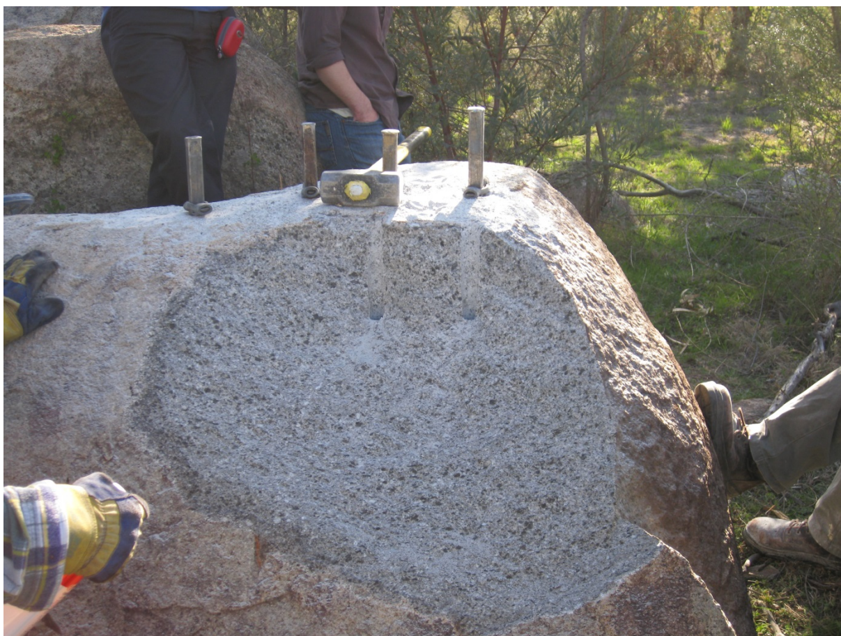
Figure 1.1 A ‘suitable rock’: In situ monzonite outcrop, Tharwa, ACT, across the road from the deeply weathered and fractured outcrop in Figure 1.2. Note the fresh rock and lack of a deeply weathered rind and fractures.
