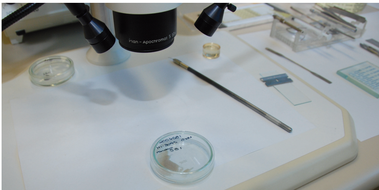
Figure 9.1 Zircon grains being handpicked in a Petri dish with ethanol.
