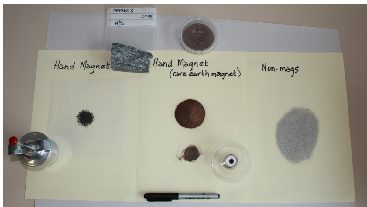
Figure 7.1 Hand magnet and rare earth magnet separation after Wilfley Table.
