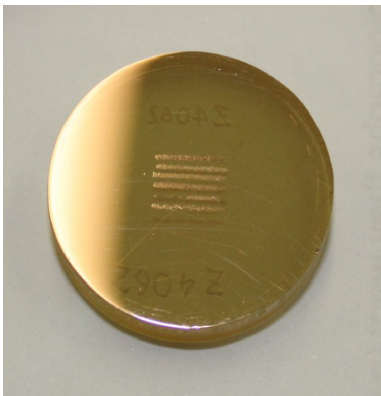
Figure 10.1 SHRIMP mount after gold coating and analysis (note surfaces scratches around the edge from the SHRIMP mount holder). Diameter of mount is 25 mm, grain rows are approximately 7 mm length x 0.4 mm width, placed within the 10 mm x 10 mm SHRIMP analytical area.
