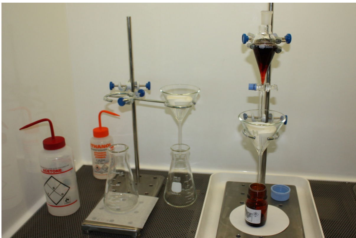
Figure 8.1 Heavy liquid separation set-up using diiodomethane (SG 3.3) in a down-draft fume cupboard.
