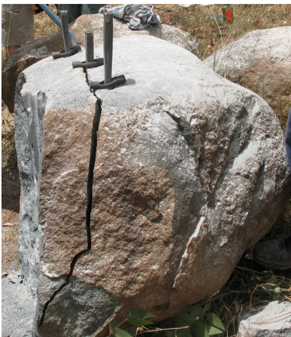
Figure 1.4 Drilling the first row of holes in the boulder from Figure 3 (top left); Splitting off the face of the rock (top right) with second row of holes visible to the right of the feathers and wedges; Splitting the second layer (bottom left); Breaking the rock into manageable pieces with a sledge hammer (bottom right).
