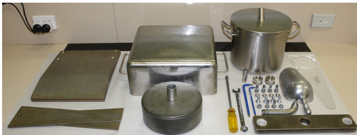
Figure 5.6 Removable components of Crushing Room 1 Boyd Jaw Crusher and Continuous Ring Mill.
