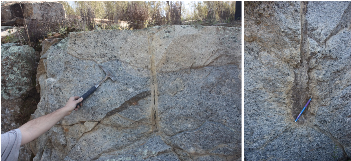
Figure 1.2 A 'less suitable rock': In situ monzonite outcrop, Tharwa, ACT. Note the deep weathering from the top of the outcrop (left) and weathering along fractures (left and right).
