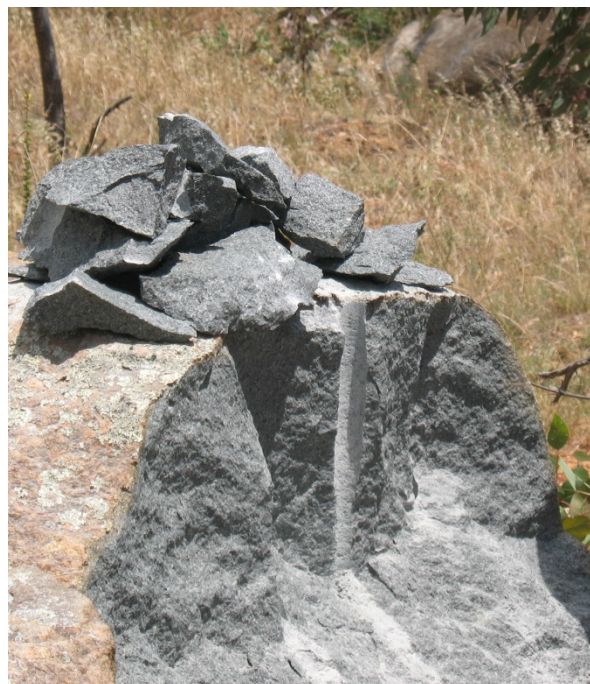
Figure 1.4 Drilling the first row of holes in the boulder from Figure 3 (top left); Splitting off the face of the rock (top right) with second row of holes visible to the right of the feathers and wedges; Splitting the second layer (bottom left); Breaking the rock into manageable pieces with a sledge hammer (bottom right).
