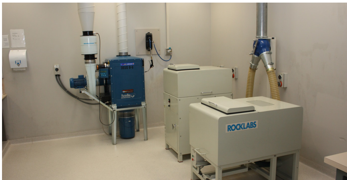
Figure 5.1 Crushing room 1: L–R dust extractor, Continuous Ring Mill and Boyd Jaw Crusher.
