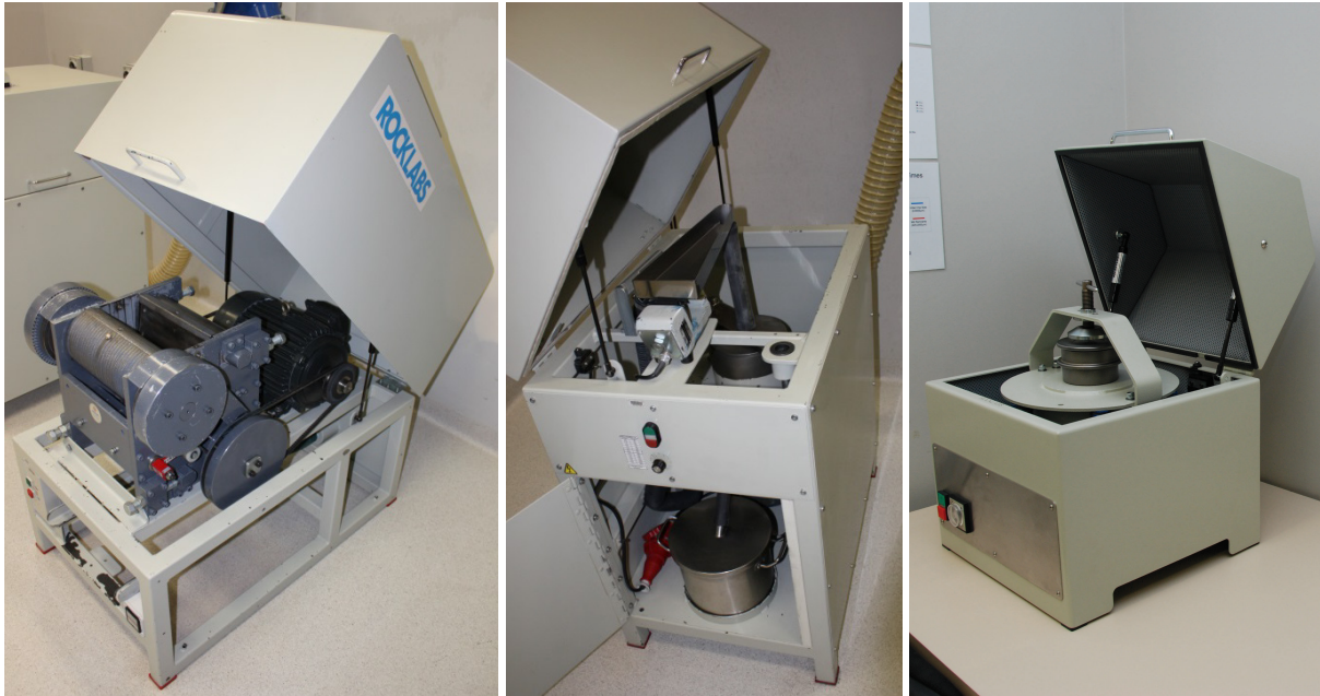
Figure 5.2 Crushing Room 1: Boyd jaw Crusher (left), Continuous Ring Mill (centre), Rocklabs Shatter Box (right).
