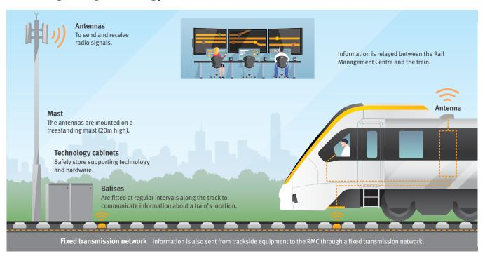
Designed for rail coverage only, the radio system uses European Standard GSM-R technology. GSM stands for Global System for Mobile Communications and the R in GSM-R stands for Railway. GSM-R is not new. In fact, it has been used for more than 20 years.
