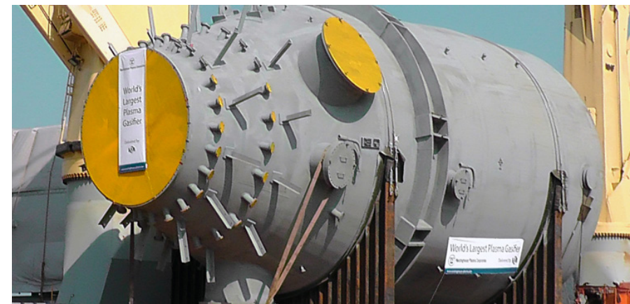
FIGURE 85: WORLD'S LARGEST PLASMA GASIFIER BEING DELIVERED TO TEES VALLEY RENEWABLE ENERGY FACILITY (SOURCE: WESTINGHOUSE PLASMA CORPORATION)
