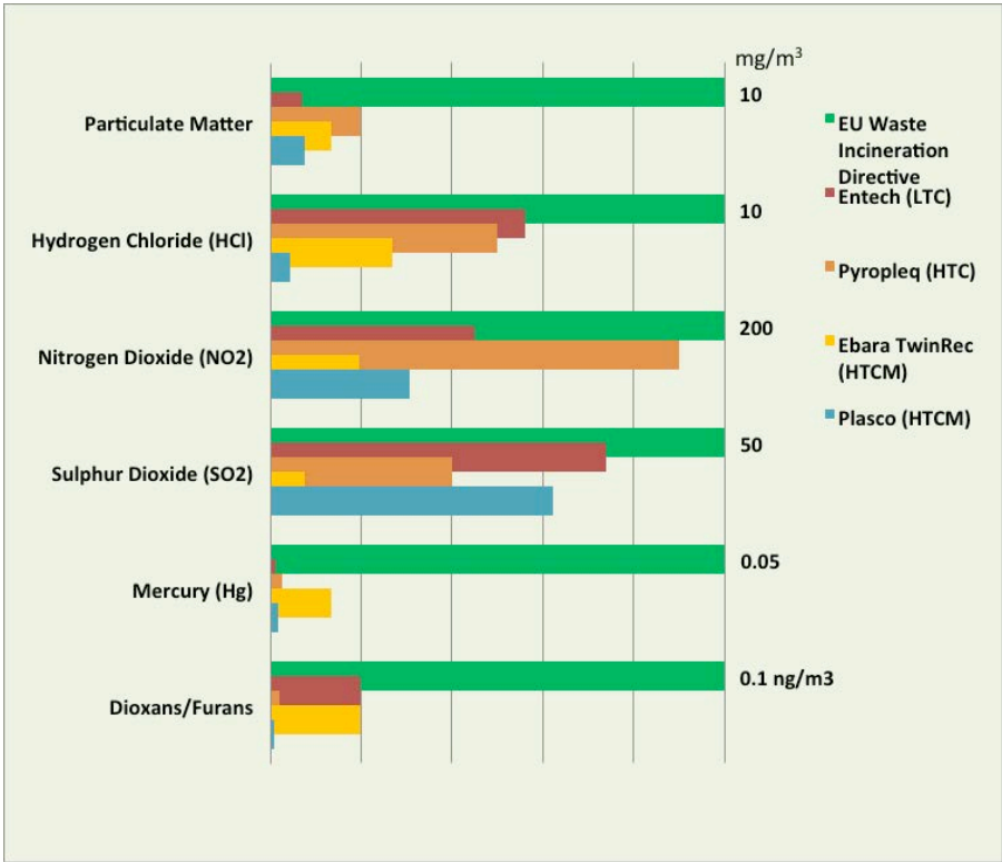
FIGURE 60: EVALUATION OF EMISSIONS FROM THERMAL CONVERSION TECHNOLOGIES PROCESSING MUNICIPAL SOLID WASTE AND BIOMASS (SOURCE: TALENT WITH ENERGY AND ONTARIO MINISTRY OF ENVIRONMENT)
