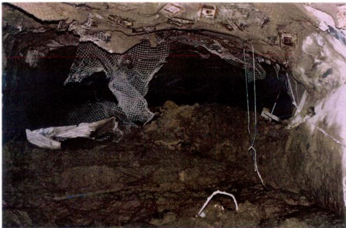
18 March 1996 3 Haulage EPD North of Fuel Store (looking north) Showing fill flow Consistency of fill * Foreground - Sloppy * Rear - Firm and putty like
