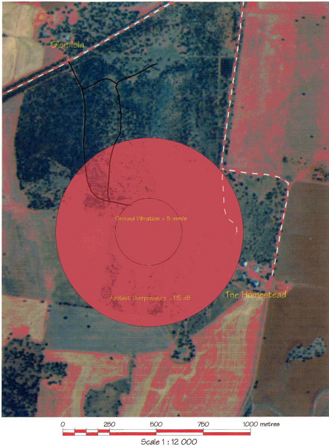
Figure 7: Contours for Airblast and Ground Vibration
