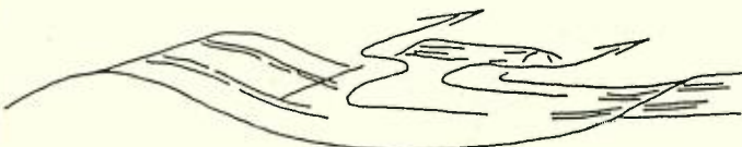
Figure 4. The bank of earth resulting from the spillway clearing can be left to act as a silt trap and water spreader.
