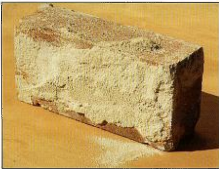
18. In earlier days lime mortar was used extensively in construction in Newcastle and other Australian cities and towns. The low strength of this mortar contributed to many losses. Similar problems with lime mortar were identified after the Adelaide, 1954 and Picton, 1973 earthquakes. (Photograph by courtesy of the GIO (NSW))
