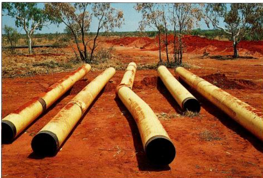
10. Damaged portions of the natural gas pipeline which extends from production fields west of Alice Springs to Darwin. The pipeline was shortened by almost one metre where it crossed the faultline. (Photo by courtesy of K. McCue, Australian Seismological Centre, Bureau of Mineral Resources)
