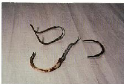
30. The failure of wall ties was a common cause of damage in older buildings in Newcastle. Most wall ties are made of 3.5 mm soft galvanised wire which corrodes readily in coastal environments. (Photograph by courtesy of the GIO (NSW))
