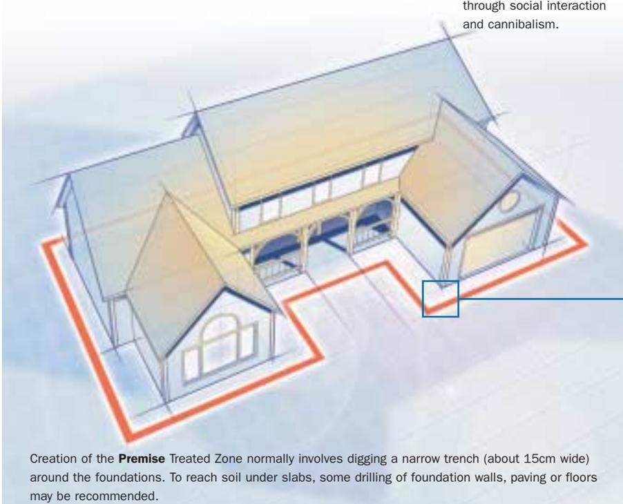
Creation of the **Premise** Treated Zone normally involves digging a narrow trench (about 15cm wide) around the foundations. To reach soil under slabs, some drilling of foundation walls, paving or floors may be recommended.
