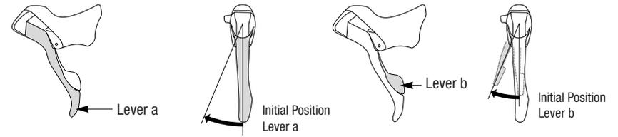
If the lever movement does not produce a complete change of chain sprocket, the lever must be moved again by amount (X') in order to execute the missing lever movement distance (X) and thus the gear shift.
