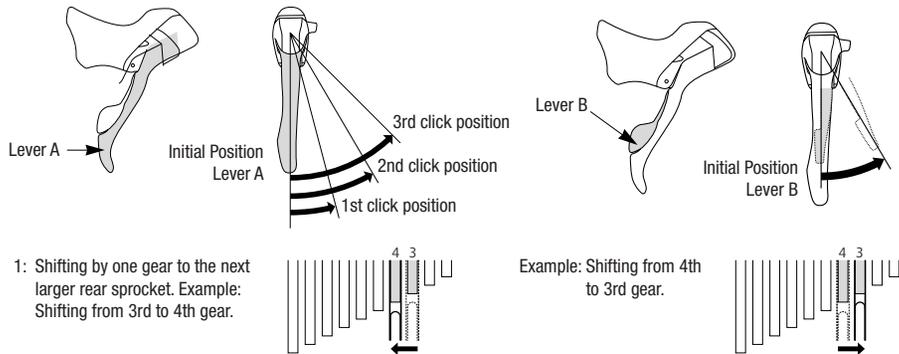
1: Shifting by one gear to the next larger rear sprocket. Example: Shifting from 3rd to 4th gear.
