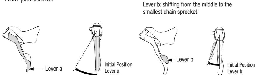
When shifting using lever b, an initial click stop marks the start of trimming (noise prevention mechanism) and a second, stronger click stop marks the complete chain sprocket shift. After trimming, the next press concludes the shift sequence.
