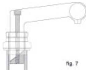
**WARNING:** On some bicycles, changing the stem or stem height can affect the tension of the front brake cable, locking the front brake or creating excess cable slack which can make the front brake inoperable. If the front brake pads move in towards the wheel rim or out away from the wheel rim when the stem or stem height is changed, the brakes must be correctly adjusted before you ride the bicycle.
