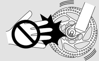
The brake saddle and the disc may be hot after braking, therefore do not touch them during or immediately after riding, as you could burn yourself. Before adjusting the brakes, check that the parts have cooled down sufficiently.
