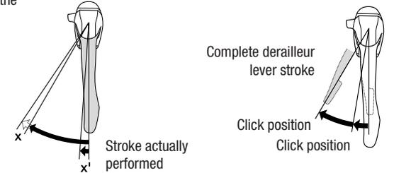
Lever 'b' moves with lever 'a' when it is actuated. However, the exertion of pressure on lever 'b' must be avoided. Correspondingly, the exertion of pressure on lever 'a' must be avoided when actuating lever 'b'. The simultaneous actuation of both levers results in no gear shift.
