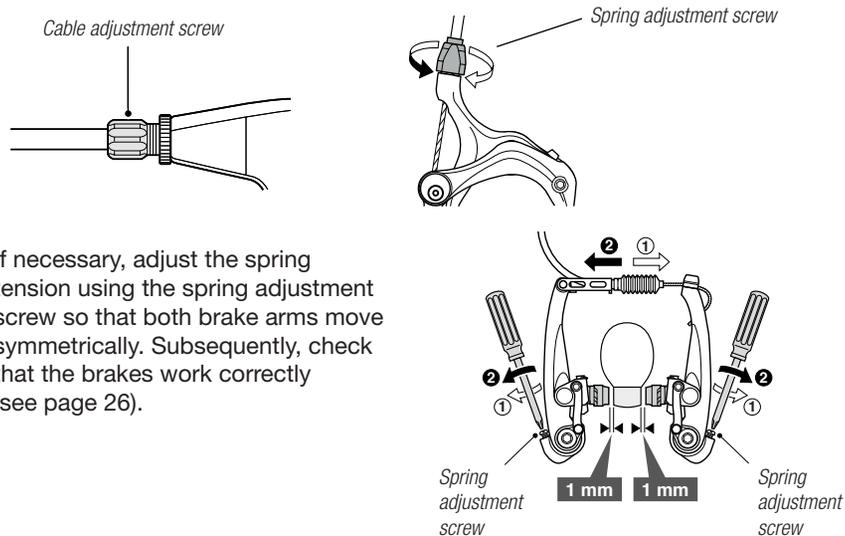
If necessary, adjust the spring tension using the spring adjustment screw so that both brake arms move symmetrically. Subsequently, check that the brakes work correctly (see page 26).
