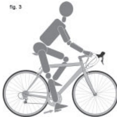
If your leg is not completely straight, your saddle height needs to be adjusted. If your hips must rock for the heel to reach the pedal, the saddle is too high. If your leg is bent at the knee with your heel on the pedal, the saddle is too low.
