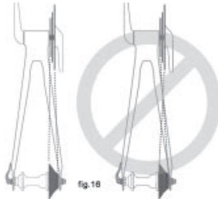
**⚠ WARNING:** Never shift a derailleur onto the largest or the smallest sprocket if the derailleur is not shifting smoothly. The derailleur may be out of adjustment and the chain could jam, causing you to lose control and fall.
