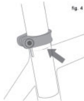
**NOTE:** Some bicycles have a sight hole in the seat tube, the purpose of which is to make it easy to see whether the seat post is inserted in the seat tube far enough to be safe. If your bicycle has such a sight hole, use it instead of the "Minimum Insertion" or "Maximum Extension" mark to make sure the seat post is inserted in the seat tube far enough to be visible through the sight hole.
