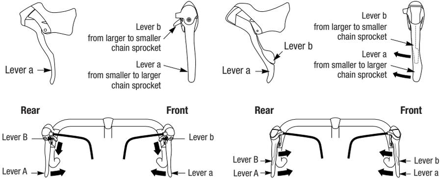
**Lever A:** Shifting to a larger rear sprocket
