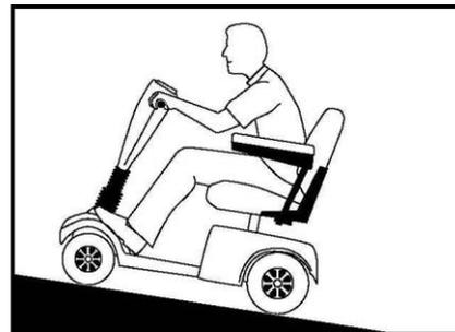
**Figure 8. Increased Stability Driving Position**
