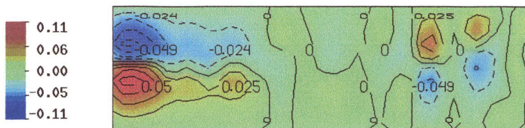
Figure 4.7 \omega (mm/s) in \sigma co-ordinates, using absolute minimum value of integration from top and bottom methods
